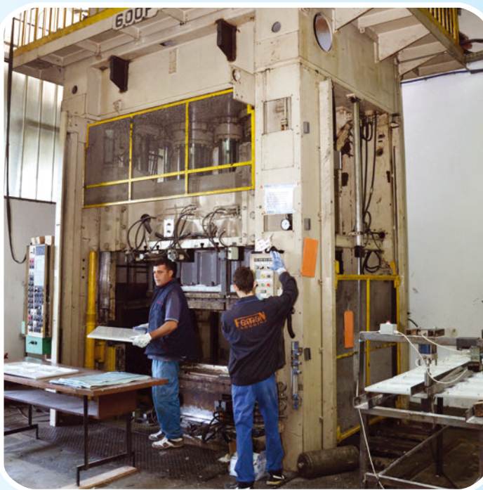
Plant with seven vertical modern hydraulic presses from 200 to 1000 tons.
